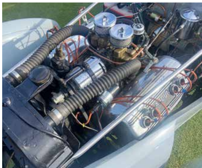
The TASCO features a 1947 Mercury V-8 engine modified with an Ardun overhead cam conversion good for 150 horsepower. The car has a three-speed manual transmission and push-button start.
